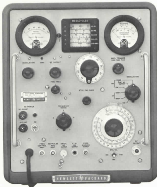
Figure 3. HP 608F Signal Generator provides up to 0.5 volt from 10 Mc to 455 Mc with the ability to be phase locked to the HP 8708A Synchronizer. Drastic reduction of drift and microphonics with phase lock eliminates a large source of error when testing high slope or narrow-band circuits. Linear FM and PM is also possible when phase locked, opening new areas of application.
